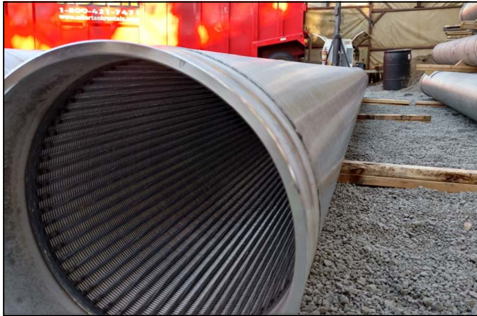
14-inch 316L Stainless Steel Well Screen
